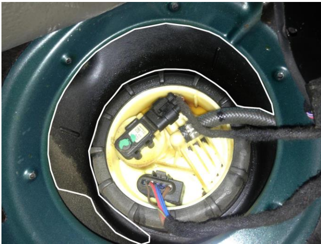
Figure 3 (Fuel residue outlined)
