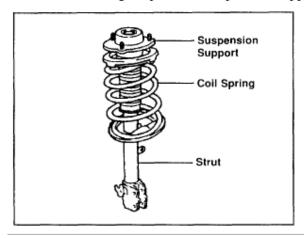
**NOTE** The rubber bushing shape of the suspension support has been changed.
