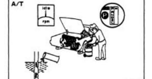
(c) With the engine OFF, add new fluid through the dipstick tube.
