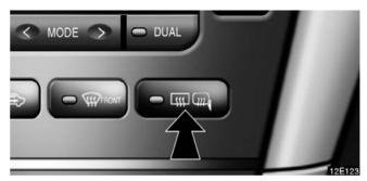
To turn the electric rear window and outside rear view mirror defogger on, push the switch.
