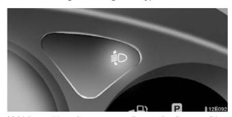
Vehicle position changes according to loading condition, passengers getting on and off, vehicle acceleration and deceleration, etc. However, as the headlight beam level is always maintained automatically by the system at the proper level, your headlights do not dazzle other road users.
