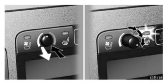
To turn on the seat heater, push the knob to pop it out and then turn the knob clockwise. The indicator light (yellow) comes on.
