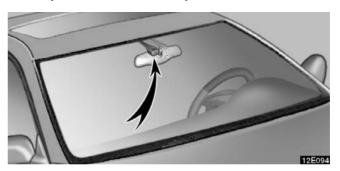
The sensor is on the inside of the windshield as shown above. Even if the wiper lever is in the "AUTO" position, the system will switch to intermittent operations in the following conditions:
