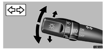
For signaling turns, move the lever up or down in the conventional manner.
