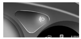
Vehicle position changes according to loading condition, passengers getting on and off, vehicle acceleration and deceleration, etc. However, the headlight beam level is always maintained automatically by the system at the proper level so that your headlights do not dazzle other road users.
