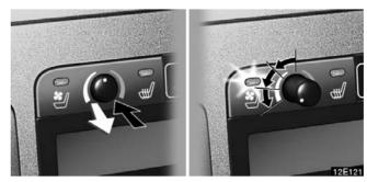
To turn on the seat ventilator, push the knob to pop it out and then turn the knob counterclockwise. The indicator light (green) comes on.
