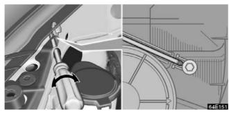
2. Turn the vertical movement adjusting bolt 2 the same number of turns and in the same direction at step 1 using a Phillips-head screwdriver.
