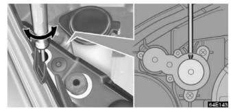
1. Turn the vertical movement adjusting bolt 1 in either direction using a Phillips-head screwdriver. At this time, keep the turning direction and number of turns in mind.
