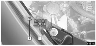
1 Vertical movement adjusting bolt 1
