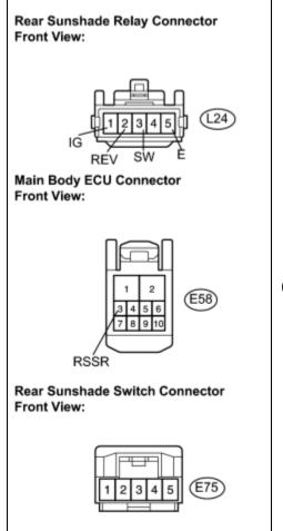
(a) Disconnect the L24 relay connector.
