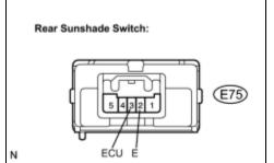
(a) Disconnect the connector from the rear sunshade switch.
