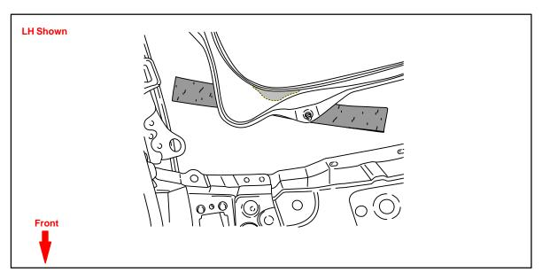
Once the felt is placed as close to the inner edge as possible, peel off the backing paper at the ends of the felt strip and stick the felt to the roof panel.
