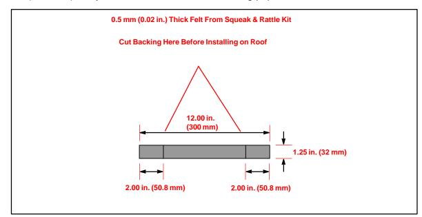
Repair Procedure (Continued) 6. Place the felt strip between the roof panel and the moon roof mounting structure panel as shown in the illustrations below.
