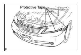
(a) Put protective tape around the front bumper assembly.
