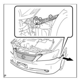
(d) Disengage the 3 claws and disconnect the front bumper assembly as shown in the illustration.
