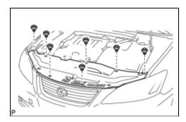
(a) Remove the 7 clips and cool air intake duct seal.
