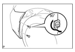
(b) Using a screwdriver, turn the pin 90 degrees and remove the 2 pin hold clips.
