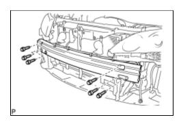
(a) Install the front bumper reinforcement with the 6 bolts.
