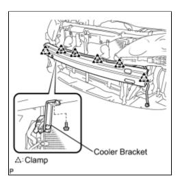
(b) Install the cooler bracket with the bolt.
