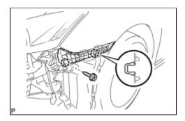
(a) Engage the 2 claws and install the front bumper stay LH.
