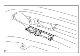
(a) Engage the 2 claws and install the No. 2 radiator grille garnish.
