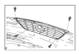
(b) Install the 2 screws and 2 clips.
