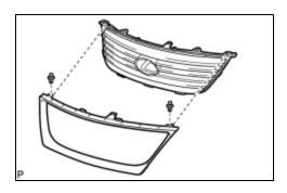
(a) Engage each claw and install the radiator grille moulding.
