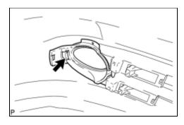
(a) Engage the claw and install the fog light bracket LH.
