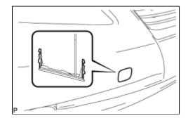
(a) Engage the 2 claws and remove the front bumper hole cover.
