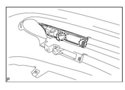
(a) Engage the 2 claws and install the radiator grille garnish.
