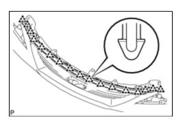
(a) Engage the 17 clips and install the radiator grille seal.
