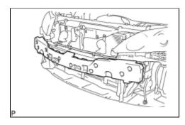
(a) Install the front bumper energy absorber to the front bumper reinforcement.
