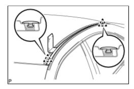
(b) Using a moulding remover, disengage the 2 clips.
