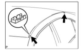
(a) Remove the 2 roof drip side finish moulding clips.
