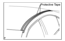
(a) Put protective tape around the roof drip side finish moulding center.
