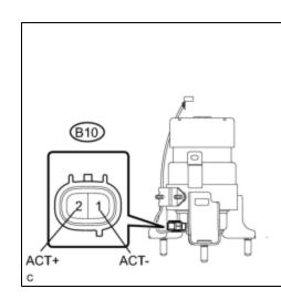
(a) Disconnect the B10 active control mount actuator connector.
