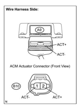
(a) Disconnect the A9 active control engine mount ECU connector and B10 active control engine mount actuator connector.
