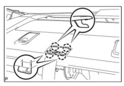
(a) Disengage the 4 claws and remove the rear seat shoulder belt hole cover.
