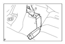
(a) Remove the bolt and disconnect the floor end of the rear seat inner with center belt assembly RH.
