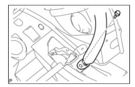
(a) Remove the bolt and disconnect the floor end of the rear seat 3 point type belt assembly LH.
