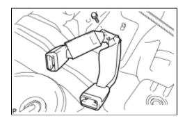
(a) Remove the bolt and the rear seat inner with center belt assembly LH.
