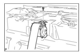
(a) Remove the bolt and the rear seat inner with center belt assembly RH.
