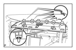
(a) Disengage the 2 clips.
