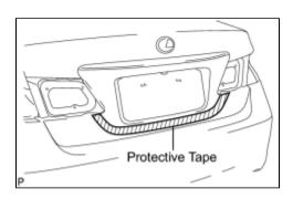
(a) Put protective tape around the luggage compartment door outside garnish sub-assembly.
