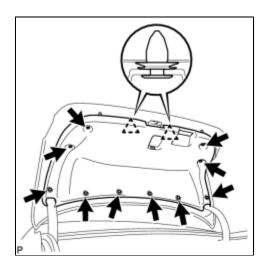
(a) Using a clip remover, remove the 10 clips.
