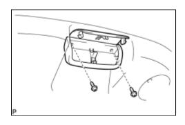
(b) Remove the 2 screws and luggage compartment door assist grip.
