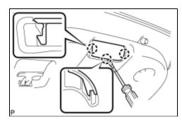
(a) Using a screwdriver, disengage the 3 claws and open the assist grip cover.
