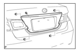
(b) Remove the bolt and 4 nuts.
