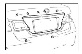
(b) Remove the 3 bolts and 4 nuts.
