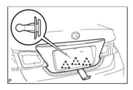
(c) Using a moulding remover, disengage the 3 clips and remove the luggage compartment door outside garnish sub-assembly.
