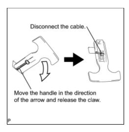
(a) Disconnect the cable as shown in the illustration, then remove the luggage compartment door inside handle.
