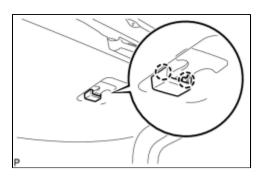
(a) Disengage the 2 claws and remove the luggage lock control cable plate.
