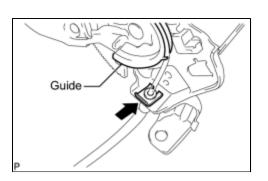
(a) Pass the No. 1 parking brake cable assembly through the guide of the parking brake pedal.
