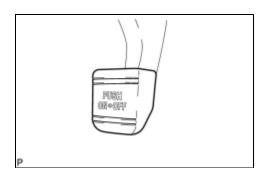
(a) Install the parking pedal pad to the parking brake pedal assembly.
