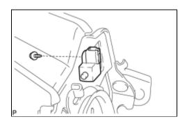
(a) Install the parking brake switch assembly with the screw.
