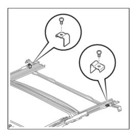
(a) Remove the 2 screws and sliding roof side stoppers.
