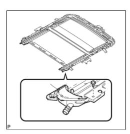
(a) Remove the screw and sliding roof piece sub-assembly LH.
