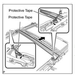
(b) Using a screwdriver, disengage the 2 claws. Then slide the sliding roof drip channel rearward to remove it.
