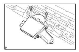
(b) Remove the 2 bolts and sliding roof drive gear sub-assembly.
