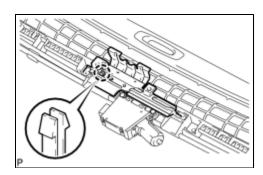
(a) Disengage the claw and remove the sliding roof room light bracket.
