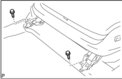
(b) Remove the 2 bolts on the front seat track bracket.
