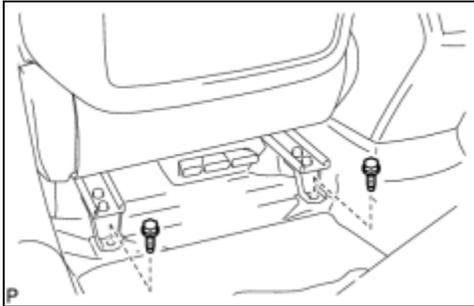
(d) Remove the 2 bolts on the rear seat track bracket.
