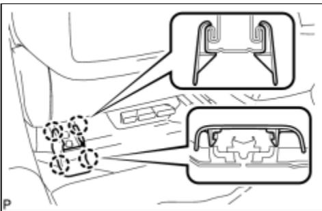
(b) Using a screwdriver, disengage the 4 claws and remove the front seat rear outer track bracket cover.
