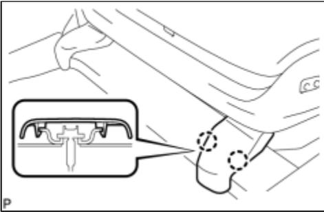
(b) Using a screwdriver, disengage the 2 claws and remove the front seat outer track bracket cover.
