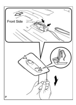
(b) Disconnect the connector and remove the spot light assembly.
