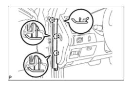
(a) Disengage the 3 claws and remove the front door opening trim cover LH.
