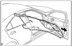
(e) Remove the roof headlining assembly from the vehicle through the front right door.
