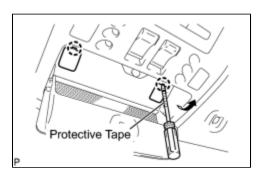
(a) Using a screwdriver, disengage the 2 claws and open the 2 covers.
