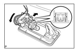
(a) Disengage the 2 claws and separate the bulb holder from the vanity light assembly as shown in the illustration.
