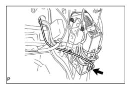
(a) Disconnect the stereo component amplifier assembly connector.
