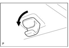
(a) Remove the visor holder by turning it counterclockwise.
