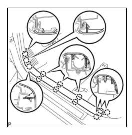
(a) Disengage the 12 claws and remove the front door scuff plate LH.
