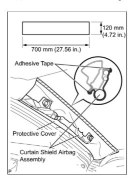
(1) Thoroughly cover the airbag with a cloth or nylon sheet and fix the ends of the cover with adhesive tape, as shown in the illustration.
