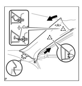
(a) Pull the upper portion of the garnish towards the inside of the cabin and disengage the 2 clips.
