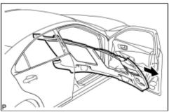
(d) Remove the roof headlining assembly from the vehicle through the front right door.
