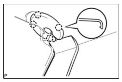
(a) Using a moulding remover, disengage the 4 claws and remove the visor bracket cover.
