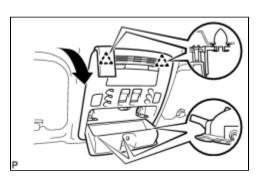
(c) Using a moulding remover, disengage the 2 clips.
