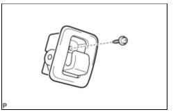
Use the same procedure to remove the coat hook on the other side.
