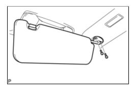
(a) Remove the 2 screws and visor assembly LH.
