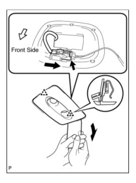
(a) Using a moulding remover, disengage the 2 clips.
