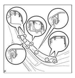
(a) Disengage the 8 claws and remove the rear door scuff plate LH.
