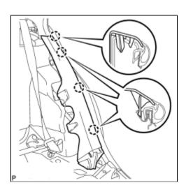
(a) Disengage the 4 claws and rear seat side garnish LH.
