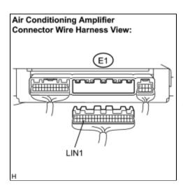
(b) Disconnect the connector from the A/C amplifier.
