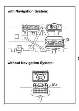
(a) Connect the connectors to the center airbag sensor assembly.
