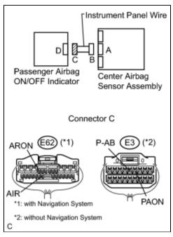
(a) Measure the resistance according to the value(s) in the table below. Standard resistance:
