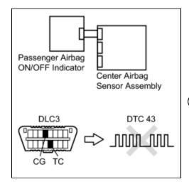
(a) Connect the connector to the center airbag sensor assembly.
