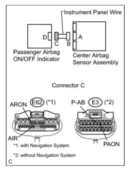
(a) Disconnect the service wire from connector B.
