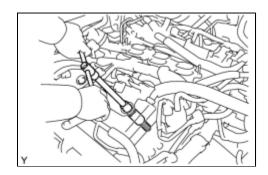
(4) Using a 16 mm (0.63 in.) plug wrench, remove the 6 spark plugs.
