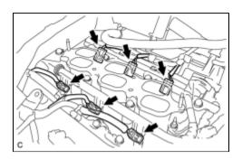
(f) Connect the 6 fuel injector connectors.
