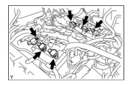
(3) Disconnect the 6 ignition coil connectors and remove the 6 bolts and 6 ignition coils.
