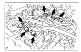
(e) Install the 6 ignition coils with the 6 bolts and connect the 6 ignition coil connectors.
