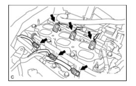
(6) Install the spark plugs to each ignition coil, and connect the ignition coil connectors.
