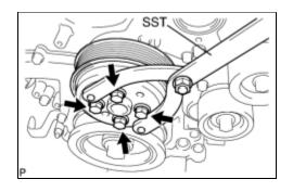
(a) Using SST, hold the water pump pulley.
