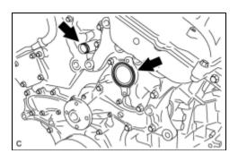
(c) Remove the water inlet housing gasket and water outlet pipe O-ring.
