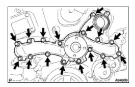
(a) Remove the 16 bolts, water pump assembly and water pump gasket.
