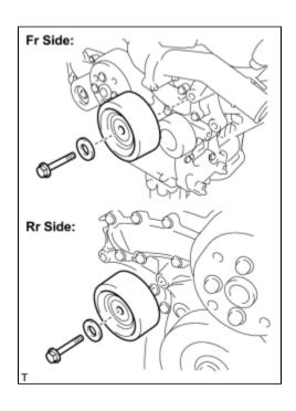
(a) Remove the 2 bolts, 2 idler pulley cover plates and 2 idler pulley sub-assemblies.
