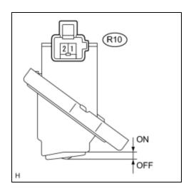
(a) Disconnect the switch connector.
