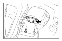
(a) Install the luggage door opening switch assembly with the 2 bolts.
