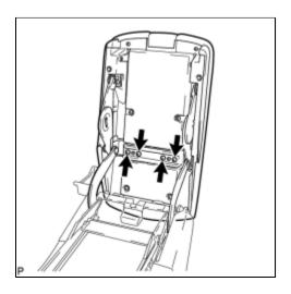
(c) Remove the 4 screws and the console compartment door sub-assembly.
