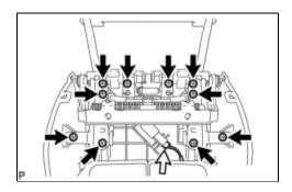
(a) Loosen the 10 screws and disconnect the connector.
