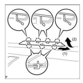
(a) Disengage the 7 claws and disconnect the center stop light set as shown in the illustration.
