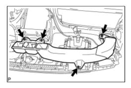
(a) Install the No. 2 heater to register duct with the 4 screws <F>.
