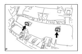
(a) Install the 2 No. 1 meter hood retainers with the 2 screws <1>.
