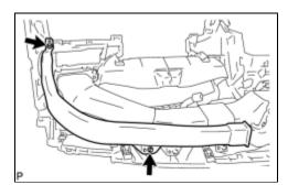
(a) Install the side No. 1 defroster nozzle duct with the 2 screws <F>.
