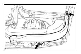
(a) Install the side No. 2 defroster nozzle duct with the 2 screws <F>.
