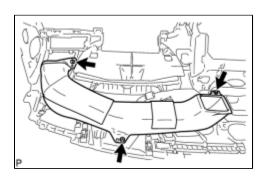
(a) Install the No. 1 heater to register duct with the 3 screws <F>.
