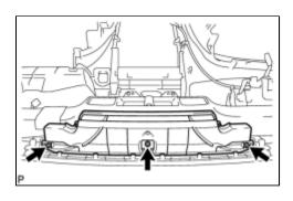
(a) Install the defroster nozzle assembly with the 3 screws <F>.
