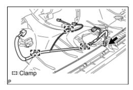
(b) Connect the connector and install the No. 3 instrument panel wire.
