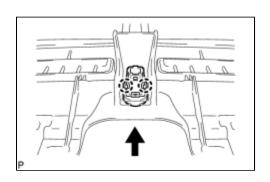
(a) Engage the 2 claws and install the automatic light control sensor.
