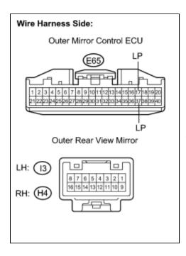
(a) Disconnect the E65 outer mirror control ECU connector.
