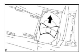
(a) Remove the No. 5 console box retainer as shown in the illustration.
