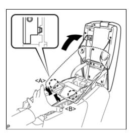
(b) Slightly deform areas <A> and <B> of the console box assembly inward to disengage the 2 claws. Next, raise the console compartment door subassembly as shown in the illustration.
