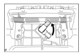
(b) Turn the console box illumination light assembly in the direction indicated by the arrow and remove it.
