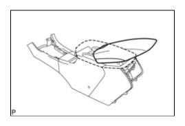
(a) Open the console compartment door sub-assembly.
