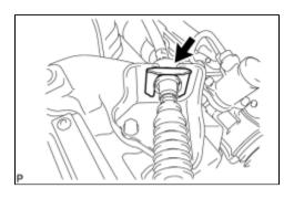
(a) Remove the clip from the transmission cable bracket.
