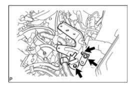
(a) Separate the wire harness clamp.
