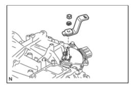
(d) Remove the nut, washer and control shaft lever from the control shaft.
