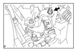
(b) Remove the nut and transmission control cable from the control shaft lever.
