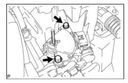
(e) Remove the 2 bolts and park/neutral position switch from the control shaft.
