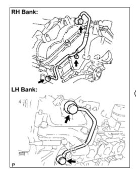
(a) Remove the oil pipe No. 1 or oil pipe assembly.
