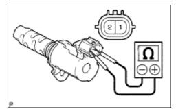
(b) Measure the resistance according to the value(s) in the table below. Standard resistance:
