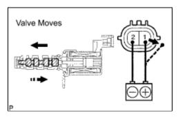
(c) Apply the positive battery voltage to terminal 1 and the negative battery voltage to terminal 2. Check the valve operation.
