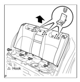
(e) Remove the 4 bolts and rear seatback assembly.
