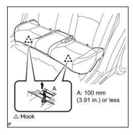
(a) Detach the 2 front hooks of the rear seat cushion assembly from the vehicle body.
