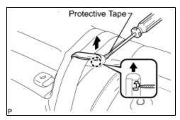
(c) Using a screwdriver, detach the claw to open the cap of the rear seat shoulder belt guide.
