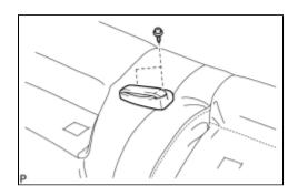
(a) Remove the 2 screws and rear seat center shoulder belt guide.
