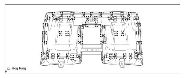
(b) Remove the 20 hog rings and rear bench type seatback cover from the seatback frame (with pad).
