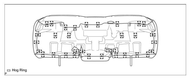
(b) Remove the 20 hog rings and seat cushion cover from the seat cushion frame (with pad).
