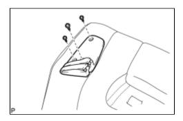
(a) Remove the 3 screws and rear seat shoulder belt guide RH.
