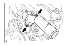
(a) Install the water inlet with the 2 nuts.
