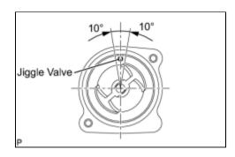
(a) Install a new gasket to the thermostat.
