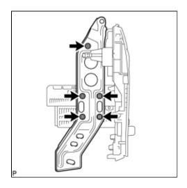
(a) Remove the 4 bolts, screw, and No. 2 radio bracket.
