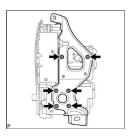
(a) Remove the 6 bolts and No. 1 radio bracket.
