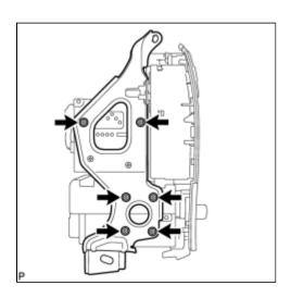
(a) Remove the 6 bolts and No. 2 radio bracket.
