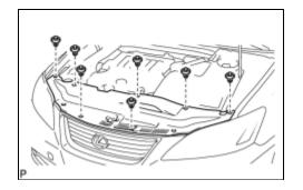
(a) Remove the 7 clips and cool air intake duct seal.
