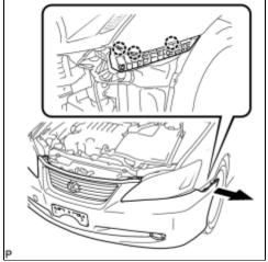
(d) Disengage the 3 claws and disconnect the front bumper assembly as shown in the illustration.
