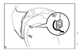
(b) Using a screwdriver, turn the pin 90 degrees and remove the 2 pin hold clips.
