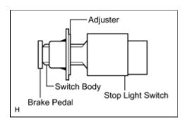
(6) Insert the switch into the adjuster until the switch body touches the pedal.
