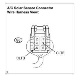
(a) Disconnect the solar sensor connector.
