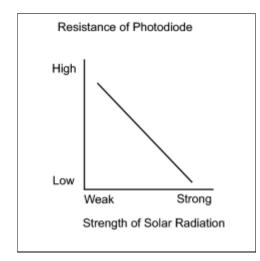
The solar sensor, which is installed on the upper side of the instrument panel, detects sunlight and controls the air conditioning in AUTO mode. The output voltage from the solar sensor varies according to the amount of sunlight. When the sunlight increases, the output voltage increases. As the sunlight decreases, the output voltage decreases. The A/C amplifier detects voltage output from the solar sensor.
