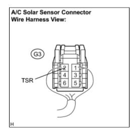
(a) Disconnect the solar sensor connector.
