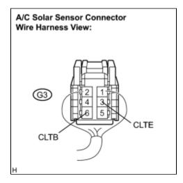
(a) Disconnect the solar sensor connector.
