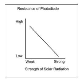
The solar sensor, which is installed on the upper side of the instrument panel, detects sunlight and controls the air conditioning in AUTO mode. The output voltage from the solar sensor varies according to the amount of sunlight. When the sunlight increases, the output voltage increases. As the sunlight decreases, the output voltage decreases. The A/C amplifier detects output voltage from the solar sensor.
