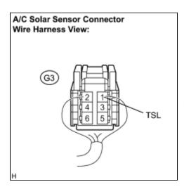
(a) Disconnect the solar sensor connector.
