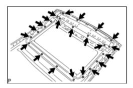
(a) Install the No. 3 sliding roof glass sub-assembly with the 22 nuts.
