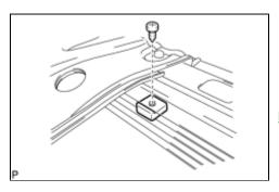
(b) Install the front sliding roof sunshade stopper LH with the screw.
