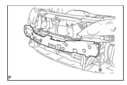
(a) Remove the front bumper energy absorber from the front bumper reinforcement.
