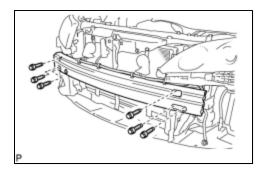
(c) Remove the 6 bolts and front bumper reinforcement.
