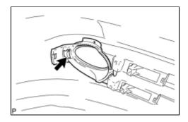
(a) Disengage the claw and remove the fog light bracket LH.
