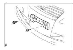
(a) Remove the 2 screws and front bumper extension mounting bracket.
