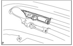
(a) Disengage the 2 claws and radiator grille garnish.
