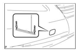
(a) Disengage the 2 claws and remove the front bumper hole cover.
