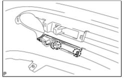
(a) Disengage the 2 claws and No. 2 radiator grille garnish.
