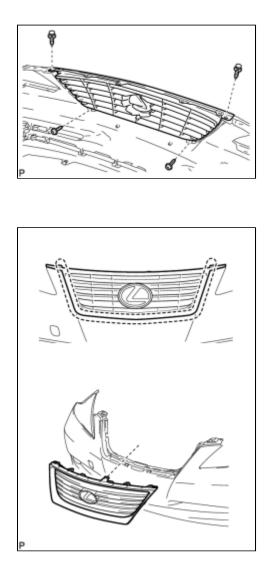
(a) Remove the 2 screws and 2 clips.
