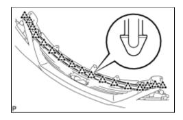
(a) Disengage the 17 clips and remove the radiator grille seal.
