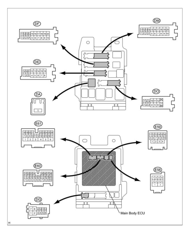
(b) Measure the resistance and voltage between each terminal of the wire harness side connectors and body ground.
