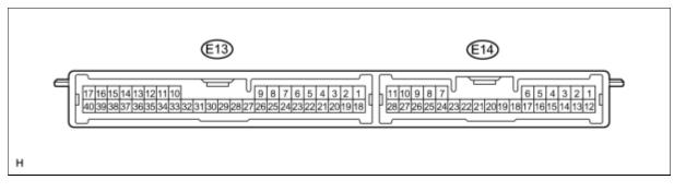
(b) Measure the voltage and resistance of the wire harness side connector.
