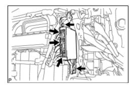
(a) Install the air conditioning amplifier assembly with the 2 bolts.
