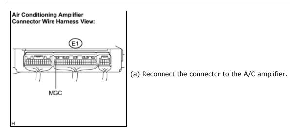
(b) Measure the voltage according to the value(s) in the table below.
