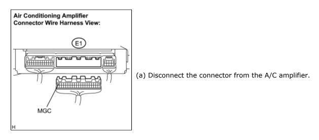
(b) Measure the voltage according to the value(s) in the table below.
