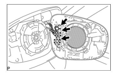
(2) Disconnect the 3 connectors and remove the outer mirror.
