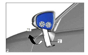
(c) Using a moulding remover, disengage the 2 claws at the lower part of the outer rear view mirror.
