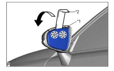
(f) Using a moulding remover, disengage the 2 claws at the upper part of the outer rear view mirror.
