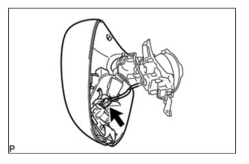
(d) Disconnect the connector and remove the No. 2 outer mirror cover with the side turn signal light assembly as a unit.
