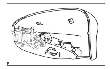
(e) Disengage the guide and remove the No. 2 outer mirror cover from the side turn signal light assembly.
