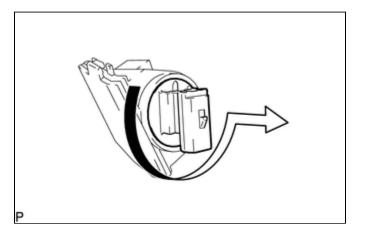
(c) Remove the outer mirror light bulb assembly from the socket.
