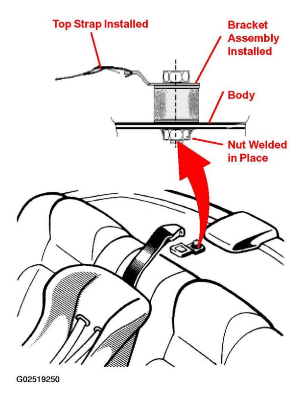
Fig. 5: Installing Bracket Assembly
