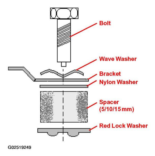
Fig. 4: Bracket Sub-Assembly
