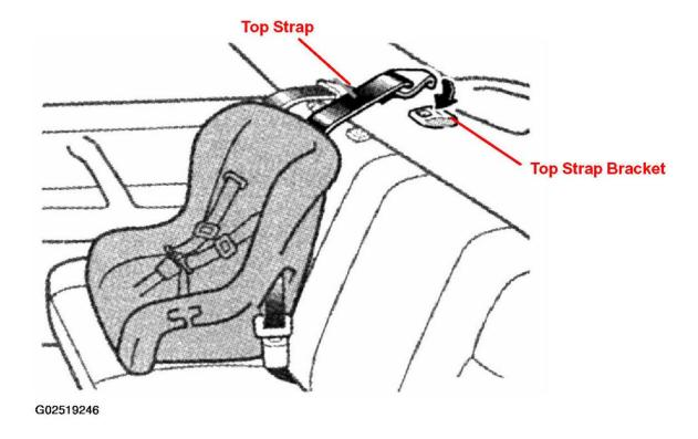
Fig. 1: Locating Top Strap Bracket Courtesy of TOYOTA MOTOR SALES, U.S.A., INC.
