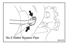
Remove the 2 nuts, and disconnect the No.2 water bypass pipe from the water pump.
