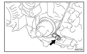
(c) Install the timing belt plate with the bolt.
