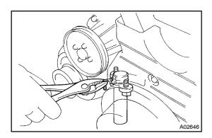
(c) Remove the 1.5 mm hexagon wrench from the tensioner with pliers.
