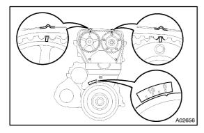
(b) Check that each pulley aligns with the timing marks as shown in the illustration.
