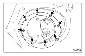
(d) Install the fuel tank vent tube set plate with the 8 bolts.
